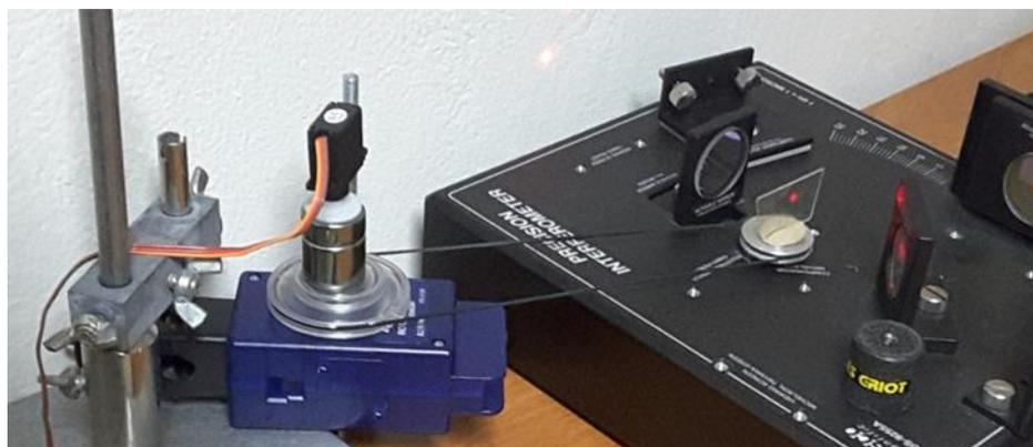
Fig.2: Photograph of the apparatus showing the belt connecting the rotation sensor pulley to the rotating stage.
