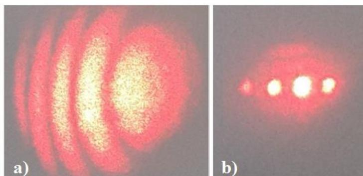
Fig. 4: The intensity fringe patterns as seen on screen a) with and b) without a laser beam enlargement lens.
