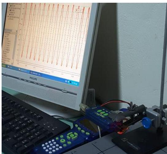
Fig. 5: Plotting the light intensity signal of the fringe pattern collected by the sensor, with respect to the angle of rotation.
