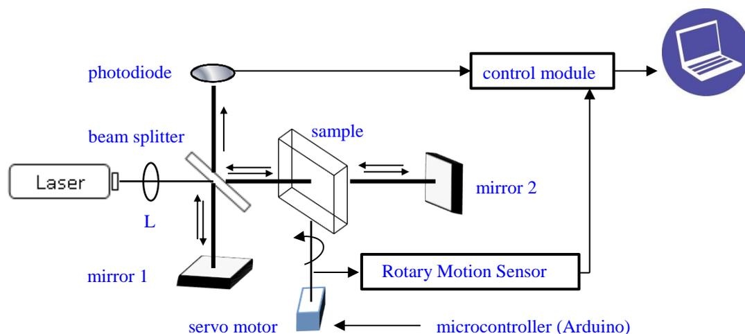
Fig.1: The setup of the automated experimental apparatus based on the interferometry of a rotating parallel plate.
