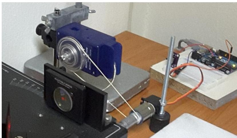
Fig.3: Photograph of the apparatus showing the servo motor as adapted to the interferometers' turning knob (micrometer) and the belt connecting it to the rotation sensor pulley.
