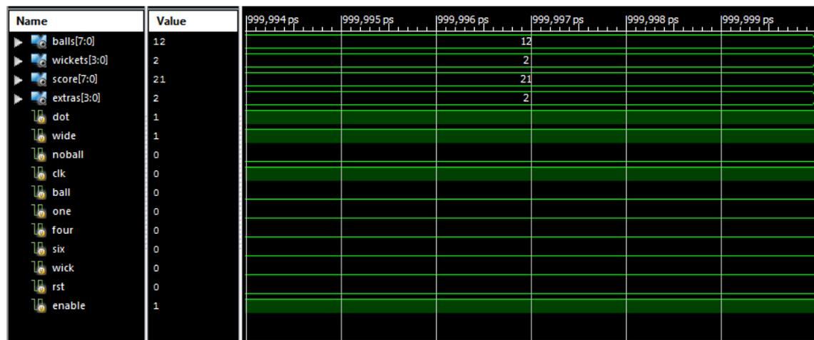
Fig.10. Timing waveforms of Final Score Displayed after completion of Game
