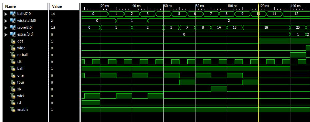
Fig.9. Timing waveforms of Display in Decimal Form
