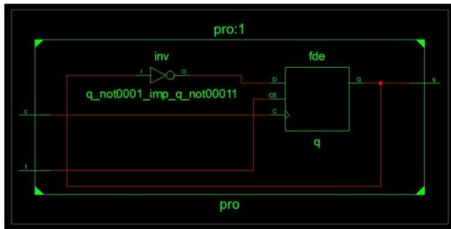
Fig.4.RTL Schematic of LFSR
