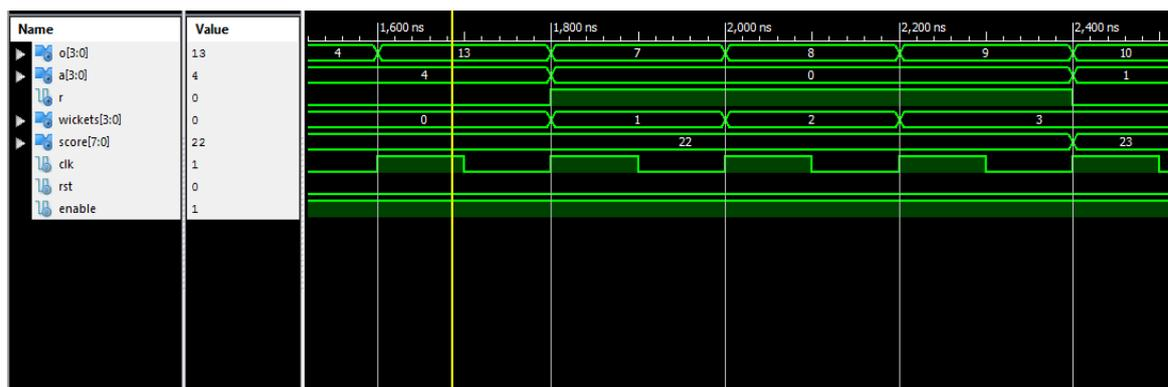
Fig.8. Timing waveforms of Game Design in Decimal Values
