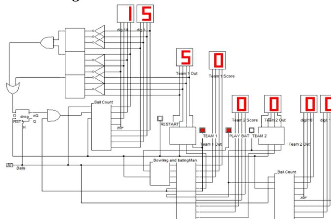
Fig .6. Gate Level Circuit Design of Game Design
