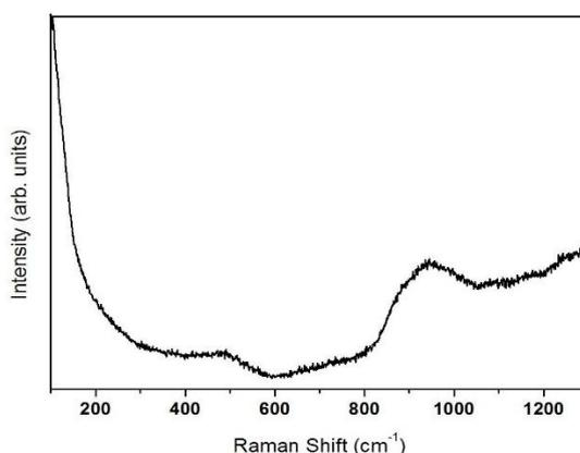
Figure 4: Typical  $\mu$ Raman spectrum of glaze of the s37 sample.
