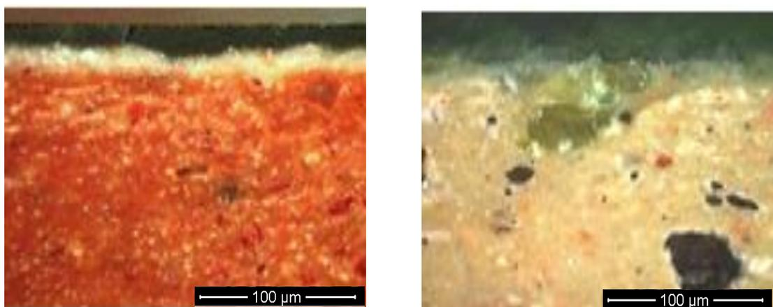
Figure 3: Microphotographs in reflected light of the cross-sections of samples collected from (a) red and (b) white clay shards. The presence of three layers glaze, slip and clay can be observed: glaze, slip and clay.
