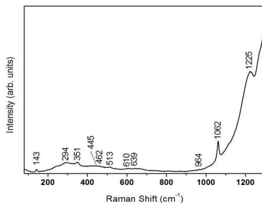
Figure 5: Typical  $\mu$ Raman spectrum of slip of the s37 sample.
