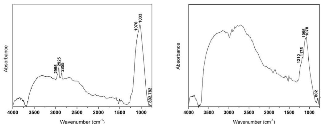
Figure 7: Typical  $\mu$ FTIR spectra of (a) glaze s37 and (b) body s37.
