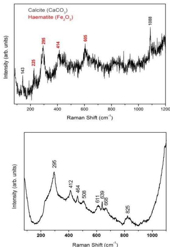
Figure 6: Typical  $\mu$ Raman spectra of (a) red s46 and (b) white type clays s51.
