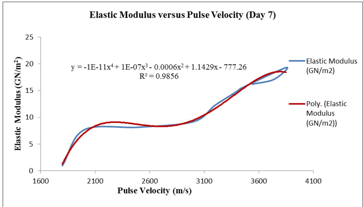
Figure 7: Graph of Elastic Modulus versus Pulse Velocity for 7-day test
