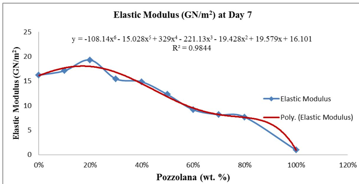
Figure 2: Graph of Avg. Elastic Modulus versus Pozzolana (wt. %) at Day 7
