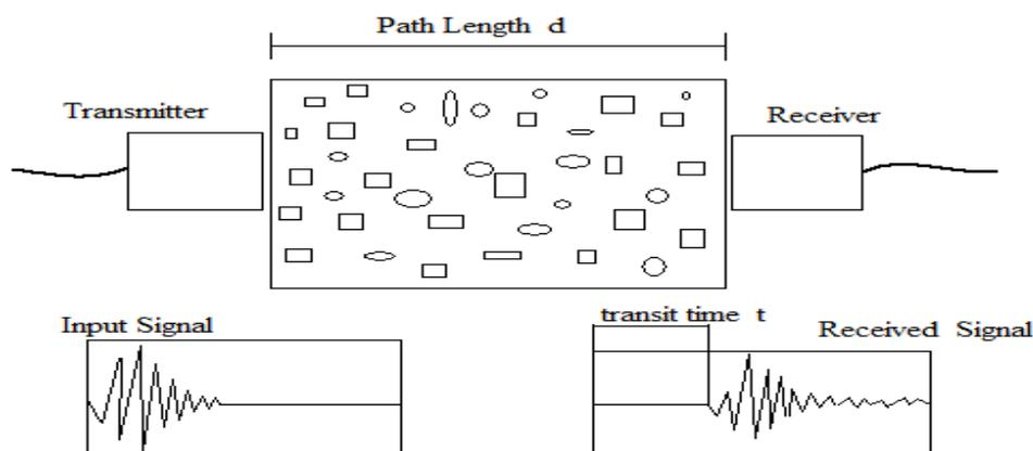
Figure 1: Ultrasonic pulse velocity testing
