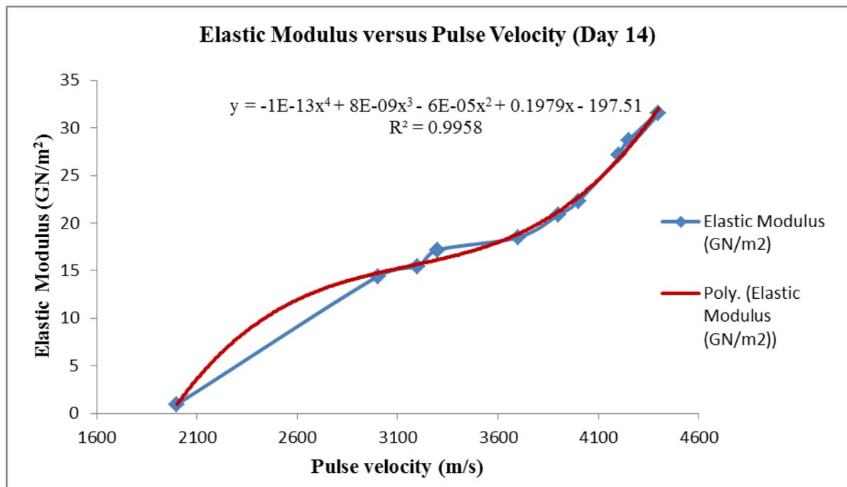
Figure 8: Graph of Elastic Modulus versus Pulse Velocity for 14-day test
