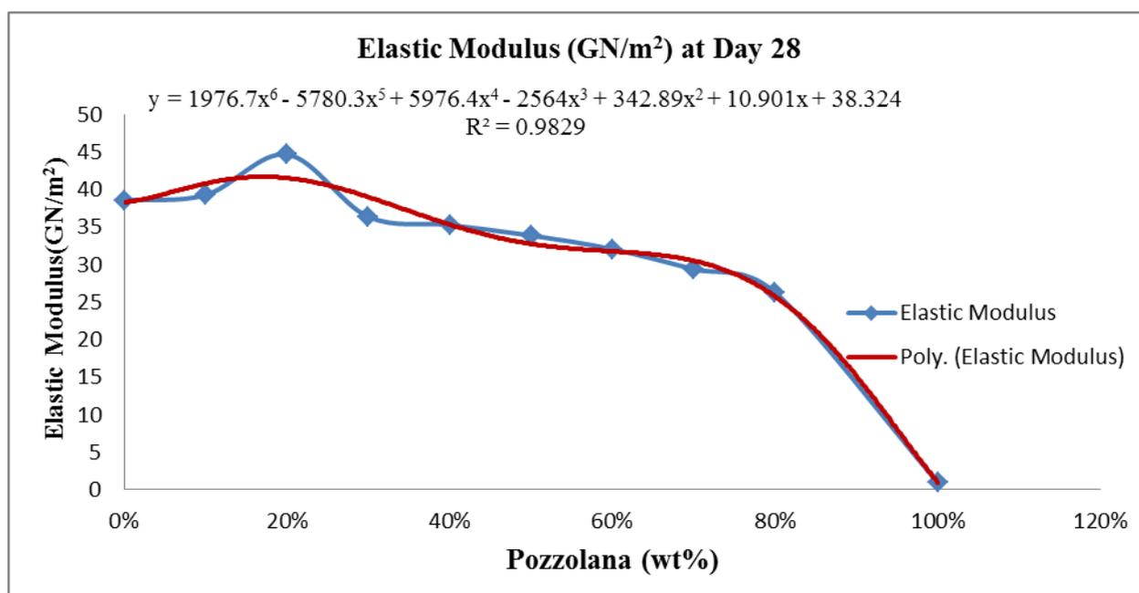
**Figure 4: Graph of Avg. Elastic Modulus versus Pozzolana (wt. %) at Day 28**
