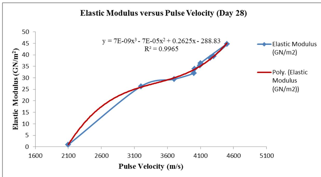
**Figure 9:** Graph of Elastic Modulus versus. Pulse Velocity for 28-day test
