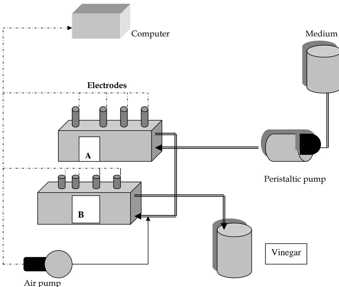
**Figure 2 Double fermentation system using the Microfermentation Cassettes.** The cassette A contains yeast in microencapsulated state. The microfermentation Cassette B contains acetic acid bacteria in immobilized state in bacterial cellulose
