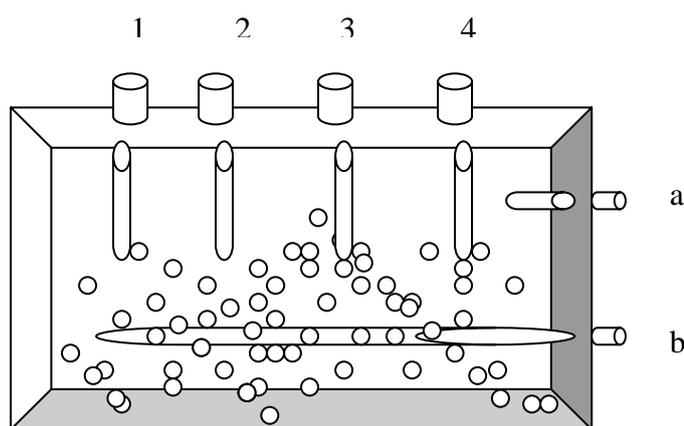
Figure 1. The Microfermentation Cassette. Ports ( 2,3), for the positions of different sensors, the air exit (4) and the temperature control (1). Ports ( a ) and ( b ) are the feed exit and entrance respectively.
