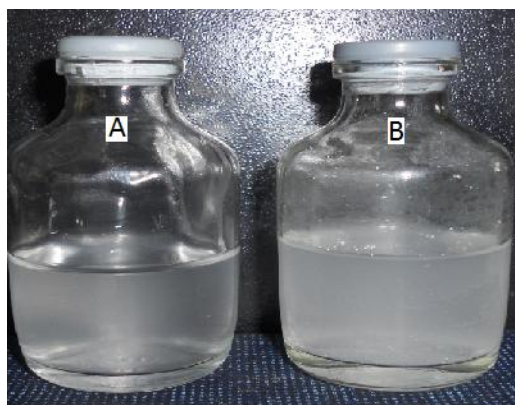
Fig. 1. Bluish white transparent nanosuspension (batch F 1 )(A), Micronized suspension of glipizide (batch F 9 )(B).
