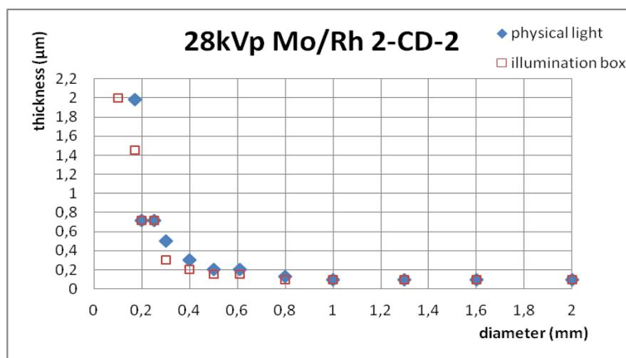
Figure 2. The film contrast detail curve for 28kVp Mo/Rh irradiation spectrum.
