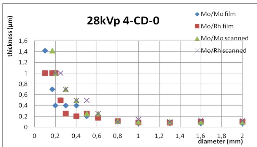
Figure 3. Contrast detail curves of films and their corresponding digitized images, for Mo/Mo and Mo/Rh filter/target combinations at 28kVp.
