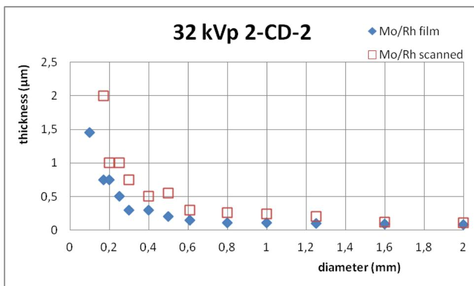
Figure 4c. Contrast detail curves of film and its digitized image, for Mo/Rh filter/target at 32kVp.
