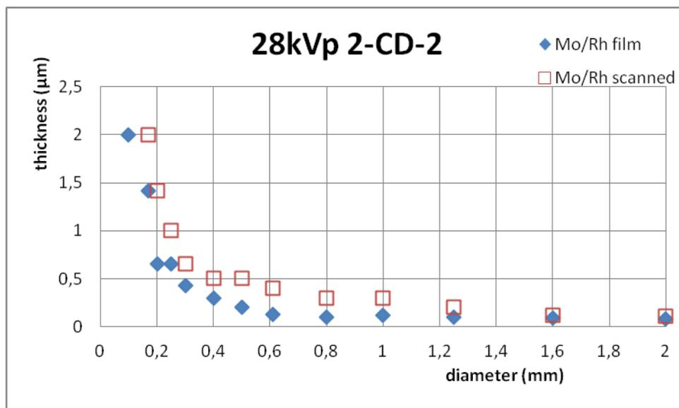
Figure 4b. Contrast detail curves of film and its digitized image, for Mo/Rh filter/target at 28kVp. The y-axis is the disk thickness and the x-axis the disk diameter.
