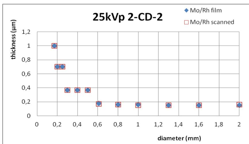
Figure 4a. Contrast detail curves of film and its digitized image, for Mo/Rh filter/target at 25kVp.
