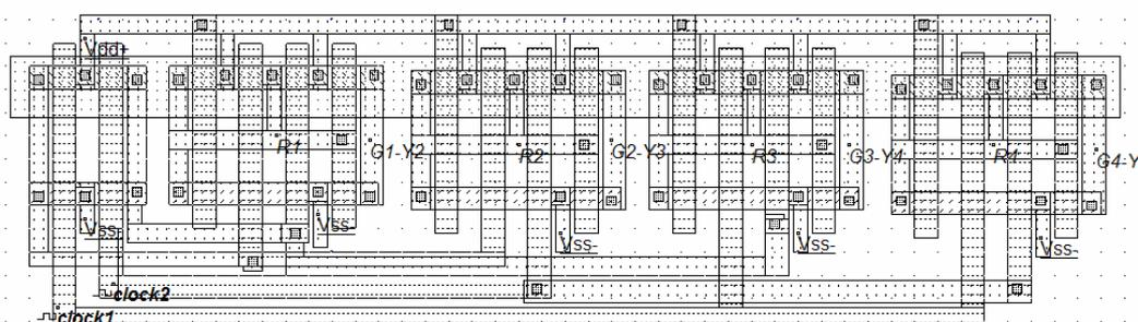
Figure-4: 90nm Technology Layout of ASIC CMOS circuit
