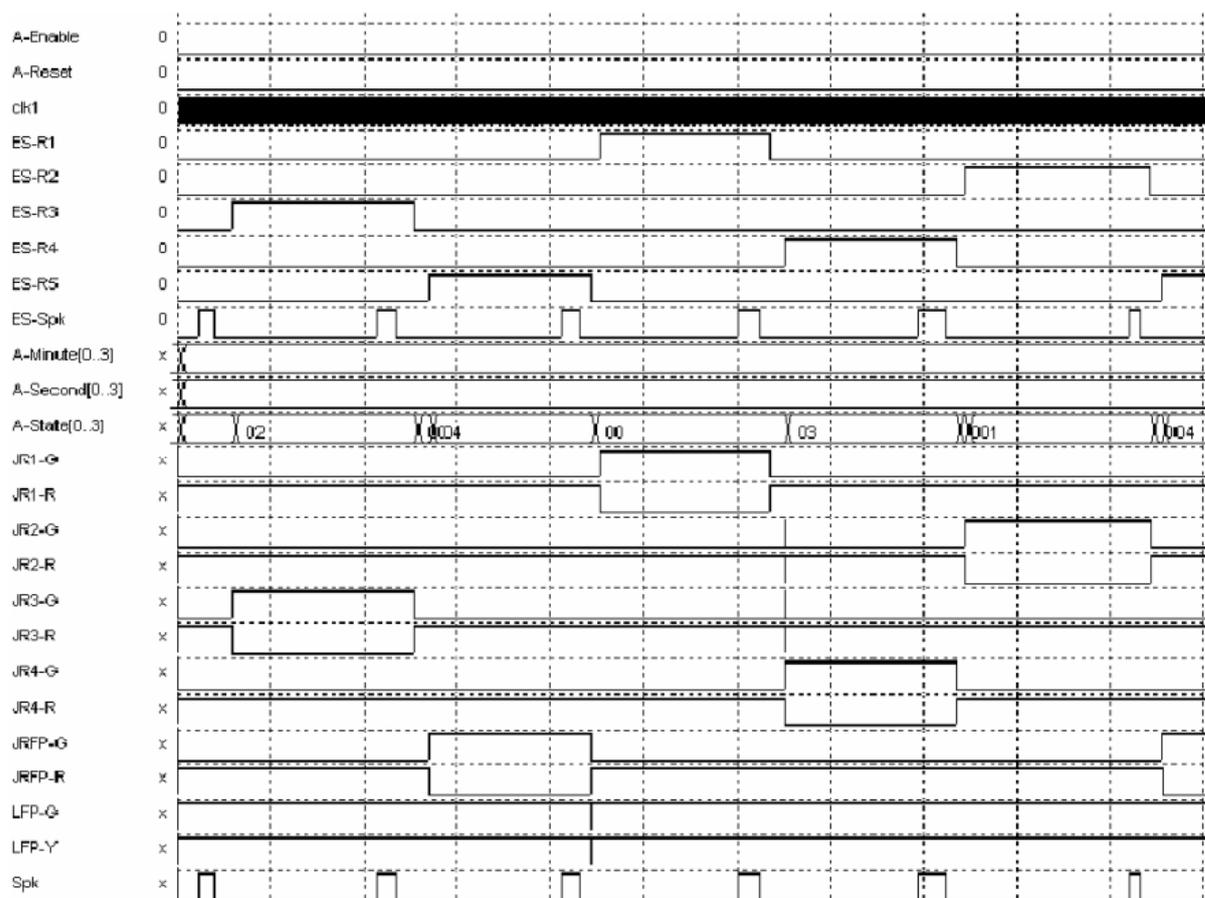
Figure – 6: Mode-2 output waveforms
