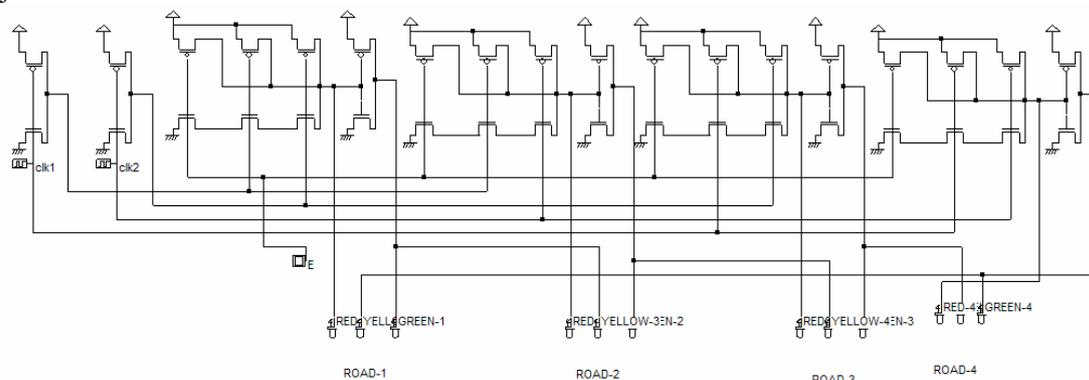
Figure-3: CMOS Signal Decoding Circuit
