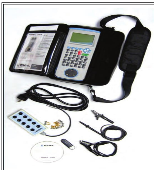
Figure 3. Rigel 288 electrical safety analyser with its carrying case, including earth bond test probe with clip, earth bond clip lead, Patient applied part module, 10 applied part adaptors, detachable 2 meter mains cable, Blue tooth USB dongle, Electronic instruction manual and removable 'quick start' card [4].
