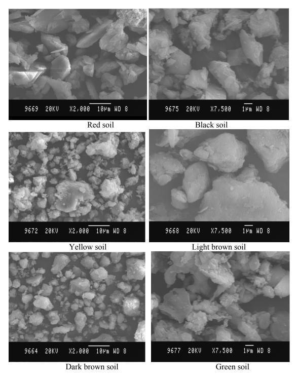
Fig.2. SEM photos of six soil samples [20]
